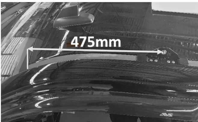
Approximate distance from rear to the centre of mounting lug(475mm)
