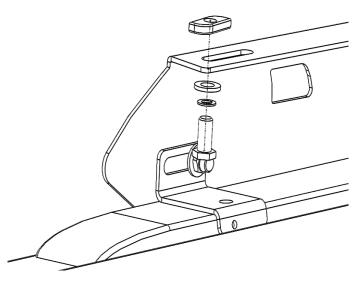
13. Place the Wedgetail Platform on the rails (Wind Deflector mounting towards the front of the vehicle), turn channel nuts 90 degree in the channel on the underside of the rack to lock into the channels. Do not tighten fully.
