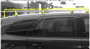
4. Mark each lug point and drill out in steps from 5mm drill bit up to 13.5mm hole to receive nutsert.
