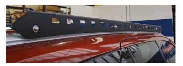
11. Fasten using 10mm nut, bolt and washer provided. Once all the hardware is ready, fasten all and repeat for the other side.
