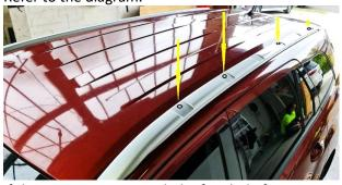
3. If there is no recess, mark the first hole from rear tailgate gap at 190mm.
