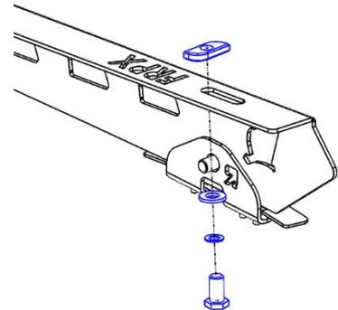
7. Place the Wedgetail Platform on the rails (Wind deflector mounting towards the front of vehicle), then spin the channel nuts 90 degree in the channel on the underside of the rack till they lock into the channels. Do not tighten fully.
