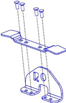
This fitment uses Structural Non-Sealed rivets for strengthening reasons
