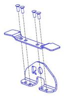
This fitment uses Structural Non-Sealed rivets for strengthening reasons Silicon must be applied to the top of the
