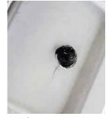
3. Locate rail on top and fasten M8 stainless bolts through the nutserts.
