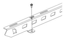
4. After fastening all the rails, fit 10mm Bolt / Split washer/ Flat washer with the channel Nuts on top of rail.
