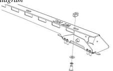
12. Place the Wedgetail Platform on the rails (Wind deflector mounting towards the front of vehicle), then spin the channel nuts 90 degree in the channel on the underside of the rack till they lock into the channels. Do not tighten fully.
