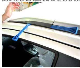
3. Remove small cover plates and remove torx bolts.
