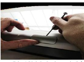
4. Remove all the visible bolts, brackets, and rails from the roof.
