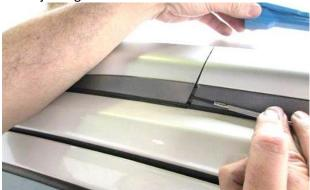
2. Remove the external plastic retainer clips from the roof rail using a trim remover as shown in the image below. Follow the same step for others as well.
