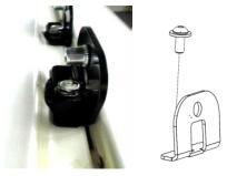
7. Fit rails to the lug using 10mm hardware (wedgetail logo facing to the front of vehicle)
