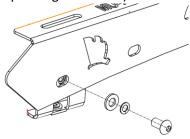
12. Fit 10mm Bolt / Split washer/ Flat washer with the channel Nuts on top of rail.\*Channel nuts to the top as shown in the diagram below
