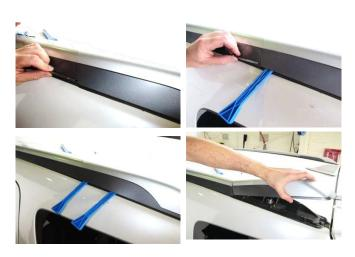
7. Remove small cover plates and remove torx Bolts.
