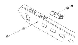
6. To secure rail to platform fit 10mm Bolt / Split washer/ Flat washer with the Channel nuts on top of rail.
