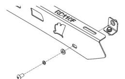
6. Fit 10mm Bolt / Split washer/ Flat washer with the channel Nuts on top of rail.
