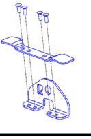
This fitment uses Structural Non-Sealed rivets for strengthening reasons
