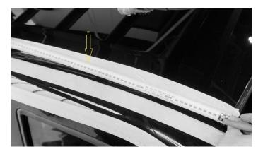
3. Mark the positions with grey lead of whiteboard marker prior removal of mastic to mount lug
