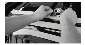
4. With a sharp knife score the vehicle paintwork either side of the mounting lug and cut down into the mastic to create a neat slot as shown in the following pictures
