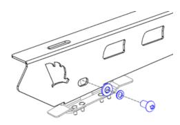
9. Fit 10mm Bolt / Flat washer/ Split washer / Strut Nuts to the top of rail.
