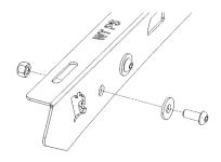
8. Using all Six Unistrut hardware, set up rail for roof rack. Three Unistrut sets per side.
