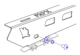
9. Fit 10mm Bolt / Flat washer/ Split washer / Strut Nuts to the top of rail.
