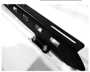
4. Fit 10mm Bolts / Split washers/ Flat washers with the channel Nuts on top of rail.
