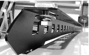
Place the Wedgetail Platform on the rails (Wind deflector mounting towards the front of vehicle), then spin the channel nuts 90 degree in the channel on the underside of the rack till they lock into the channels. Do not tighten fully.
