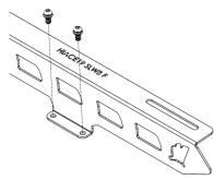
**Step 4:**Fit 10mm Bolts / Split washers/ Flat washers / Channel Nuts to the top of rail.
