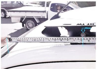
\*You should ensure the cut sections correspond with the 2 centre mounting holes in the Wedgetail rail prior cutting the channel rubber
