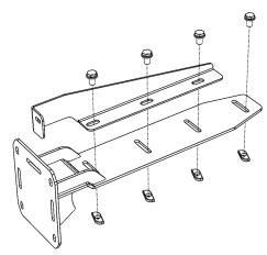
2. Fasten the M8 X 22mm Bolt and washer using a Nyloc Nut as shown below.
