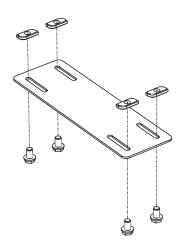
Fasten the bolt by placing the assembled bracket under the rear two crossbars. Refer to the diagram.
