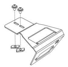
2. If using Rock Lights, assemble the attachment to Light Mount using M6 Bolt, Washer and Nyloc Nut as shown.
