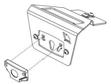
4. Assemble the bracket on the top of the cross bar using bolt, washers, and channel nuts. Refer to the diagram.
