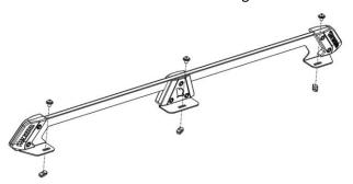
2. Fasten the Side Rails to the platform using M8 Stainless bolt and washers and channel nuts. Place the channel nuts in the cross bar and rotate 90 degrees to ensure secure fitment as shown.
