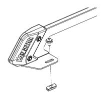
Fasten the Side Rails to the platform using M8 Stainless bolt and washers and channel nuts. Place the channel nuts in the cross bar and rotate 90 degrees to ensure secure fitment as shown.
