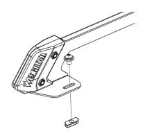
2. Fasten the Side Rails to the platform using M8 Stainless bolt and washers and channel nuts. Place the channel nuts in the cross bar and rotate 90 degrees to ensure secure fitment as shown.
