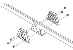
2. Loosely fasten the side rails using the M8 Bolts and channel nut. Refer to the diagram.
