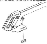
3. Fasten the Side Rails to the platform using M8 Stainless bolt and washers and channel nuts. Place the channel nuts in the cross bar and rotate 90 degrees to ensure secure fitment as shown.
