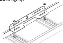
5. Insert the M8 Bolts and washer or rivets to fasten the bracket to the solar panel.
