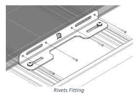
6. Adjust for desired position. Secure all the bolts and nuts.
