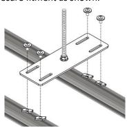
Secure wheel by passing M12 threaded rod through a wheel stud hole and fasten with wing nut and plate supplied.
