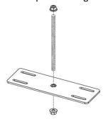
2. Fasten the Wheel Carrier Bracket to the platform using M8 Stainless bolt and washers and channel nuts. Place the channel nuts in the cross bar and rotate 90 degrees to ensure secure fitment as shown.
