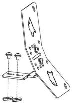
Keep a gap of 3 crossbars and then put the 2<sup>nd</sup> Trax plate on the 4<sup>th</sup> crossbar.
