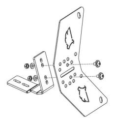
Assemble the bracket on the crossbar using M8 Bolt, washer, and channel nuts.
