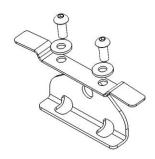
7. Attach rails to the lugs using 10mm hardware (as per diagram below). tighten.
