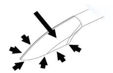
Using a flat head screw driver place in the join between the plastic cap and backing plate. Pull cover outwards untill clips let go.
