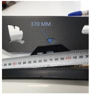
Position the Wedgetail rails in the location aligned with the marked hole and mark the 2nd hole accordingly.
