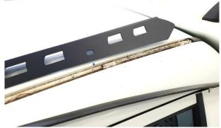
4. Place the Lug centrally aligned with the mark and mark the rivet mounting holes. Repeat the same for all other lugs.
