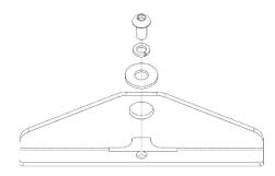
3. Attach Rails to lugs using 10mm hardware with the wedgetail logo facing to the front of the vehicle. Refer to the diagram.
