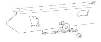
4. Fit 10mm Bolt / Flat washer/ Split washer / Strut Nuts to the top of rail.
