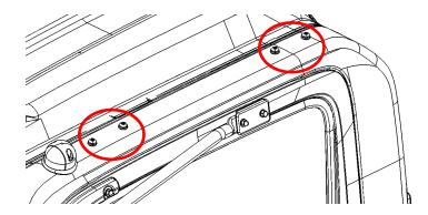
Apply silicone on all the roof channel mounting holes to prevent any water ingress.
