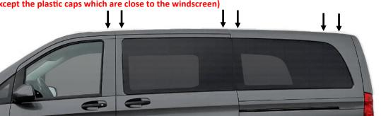
Apply silicone on all the roof channel mounting holes to prevent any water ingress.
