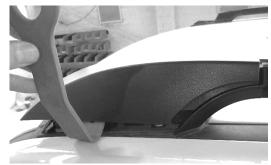
2. Remove the small plastic stops from the roof mounting threads and then remove the bolt as shown below.
